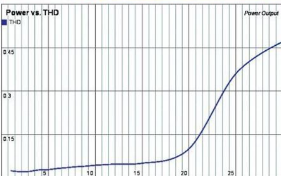
Power output vs. THD at 1 kHz into 8 ohms.
